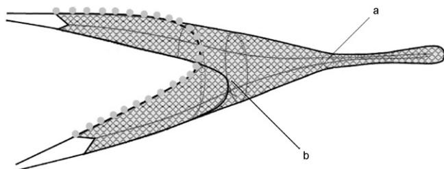
Fig. 1. Camera locations in the demersal trawl gear: (a) mouth and (b) extension. Modified from Pol (2003).
